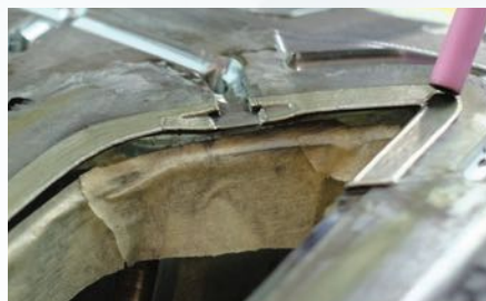
Parting line (PL) repair for material NAK80
