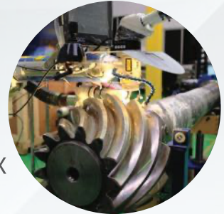
Gear shaft dimension repair welding
