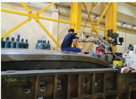
Cast Iron press die, laser welding at room temperature
