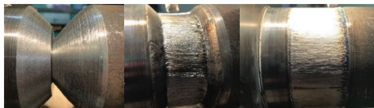
Pump shaft's butt-joining material AISI 4140/SCM440
