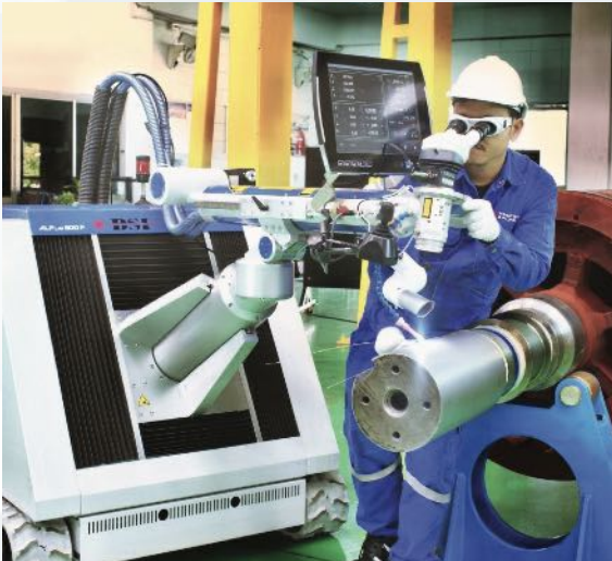
No electric arc process for motor rotor
