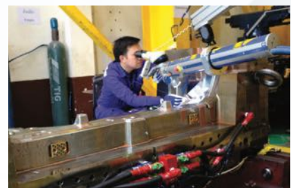
10 tons plastic injection mold, material NAK55
