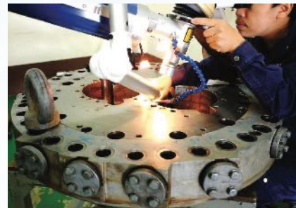
Gear shaft dimension repair welding
