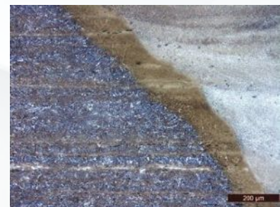
Heat-affected-zone (HAZ)-Material Duplex
